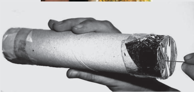
Fig. 13a and 13b: Model of the pinhole camera.
